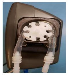
The pump head can be pulled out (the squeeze tube will come with it) and a new squeeze tube can be wrapped around the head, and the head re-installed onto the motor shaft.
