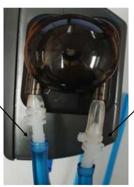
Injection Hose – goes from this side of the pump to the Injection Manifold.
