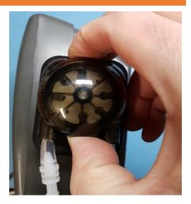
The head cover will come off to expose the squeeze tube and the head.
