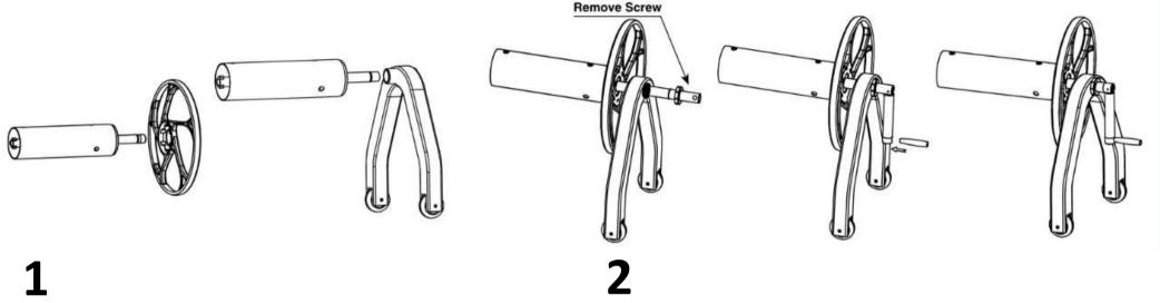
Push hand wheel onto hub ensuring they lock in. Insert Hub through roller frame – make sure the handle end is at the end with wheels
