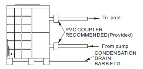
Condensation: Since the Heat pump cools down the air about  $4-5^{\circ}$ C, water may condense on the fins of the horseshoe shaped evaporator. If the relative humidity is very high, this could be as much as several litres an hour. The water will run down the fins into the basepan and drain out through the barbed plastic condensation drain fitting on the side of the basepan.
