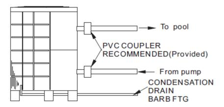
Condensation: Since the Heat pump cools down the air about 4 -5°C, water may condense on the fins of the horseshoe shaped evaporator. If the relative humidity is very high, this could be as much as several litres an hour. The water will run down the fins into the basepan and drain out through the barbed plastic condensation drain fitting on the side of the basepan.
