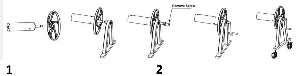
Push hand wheel onto hub ensuring they lock in. Insert Hub through roller frame
