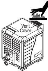
**⚠ WARNING** — **Risk of asphyxiation if exhaust is not correctly vented. Follow venting instructions exactly when installing heater.** Do not use a draft hood with this heater, as the exhaust is under pressure from the burner blower and a draft hood will allow exhaust fumes to blow into the room housing the heater. The heater is supplied with an integral venting system for outdoor installation.
